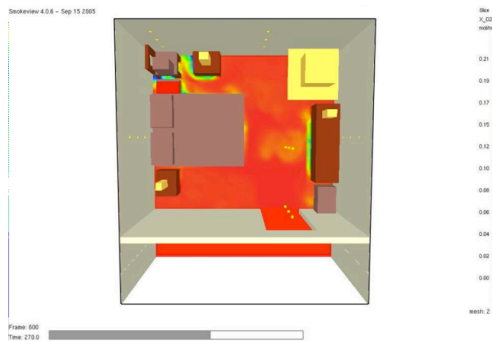
Fig. 5 - Oxygen concentration seconds before flashover
