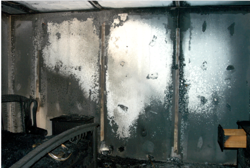
Fig. 3 Cell 3 - This fire was also set to the left of this photograph and, like Cell 2, burned for two minutes post-flashover. The ventilation flow was affected primarily by the room’s physical layout. The flow resulted in the recurring, post-flashover “V” shaped burn patterns in Cells 2 and 3. These patterns marked the most severely damaged areas in each cell. The apex of each “V” is several feet away from the fire’s origin.
