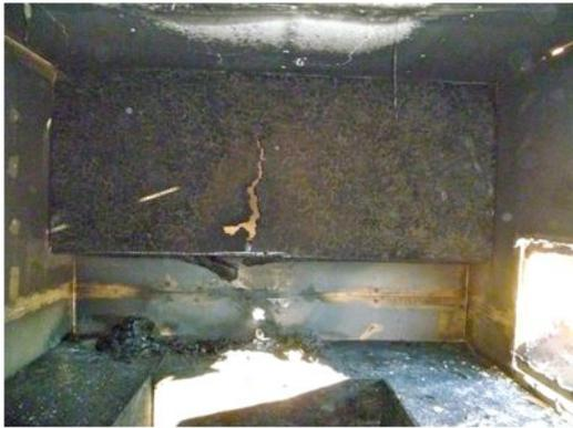
Figure 6 – View of area of origin. The pan of burning oil was on the lower cabinet
