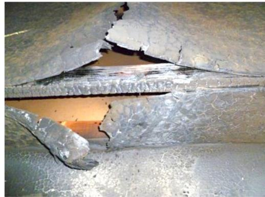
Figure 7 – Underside of cabinet directly above the origin
