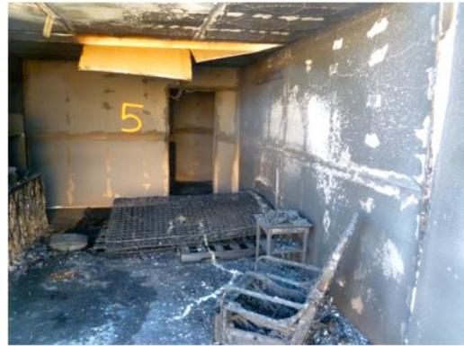
Figure 3 – Opposite end of large room showing areas with less damage. Room of origin is beyond distant doorway
