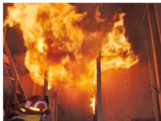
(Fig. 6) Upper layer ignites and extends well away from the compartment
